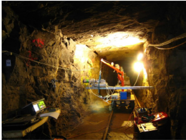
Figure 2: Pneumatically driven impulse hammer source pre-stressed against the Richtstrecke gallery wall (see Fig 1).
