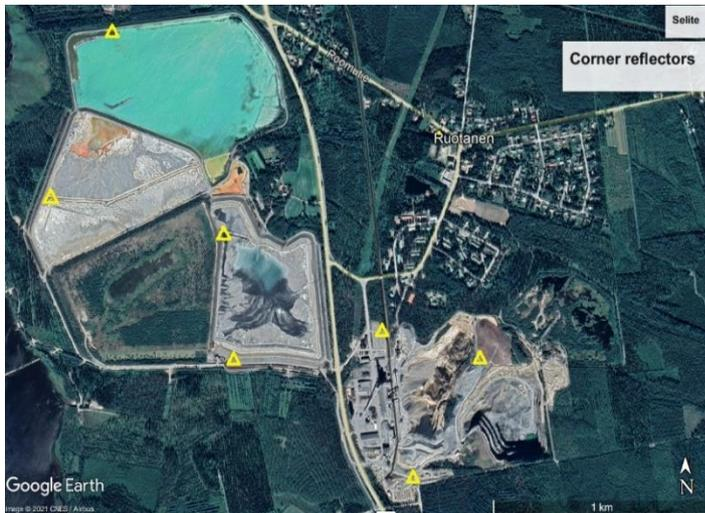
Figure 6. Pyhäsalmi mine area taken from Google Earth. Yellow triangles indicate the positions of corner reflectors designed for Copernicus earth observation satellites. The Callio Lab research activities utilise both the surface and the underground facilities.
