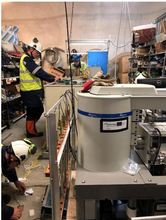
Figure 23. Lab 5 at the main level +1410 meters below surface. Neutron flux measurements with liquid organic scintillators being prepared. BSI low background HPGe gamma spectrometer also pictured.
