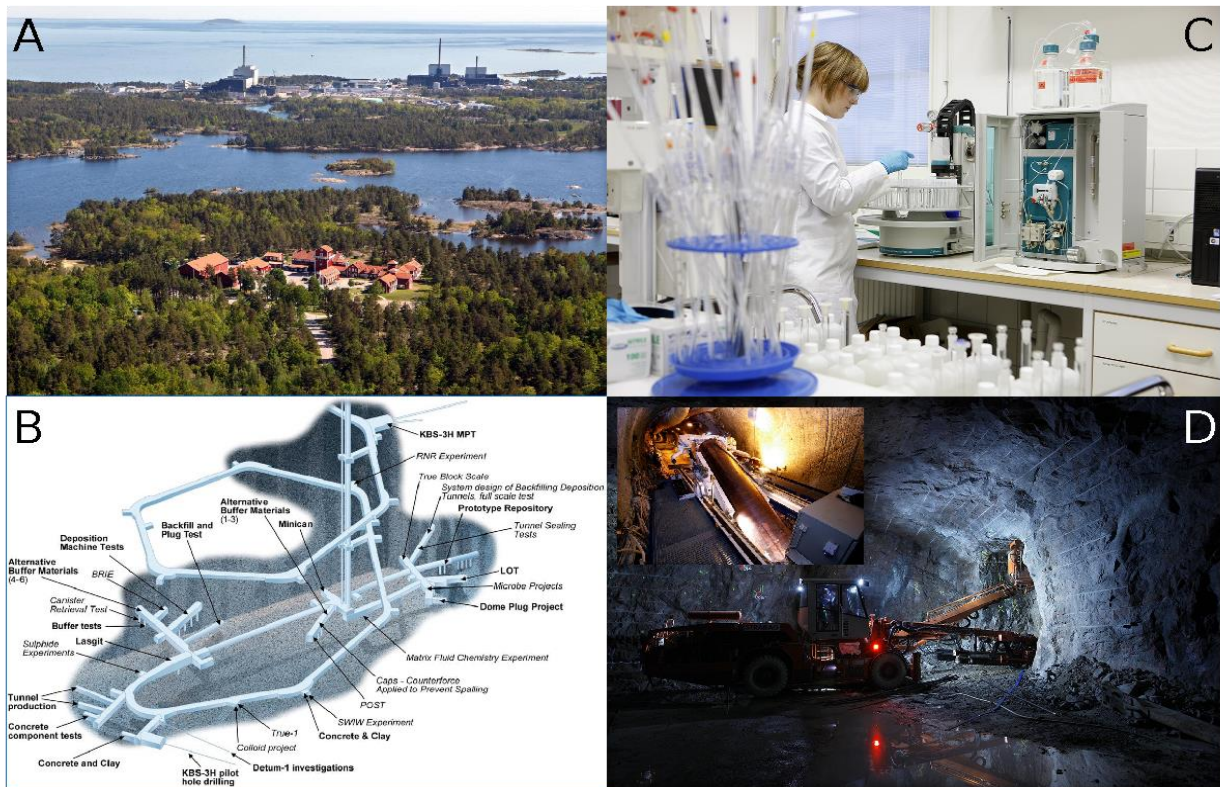
Figure 2: a) Aerial view of the Äspö HRL (red buildings), b) the underground facility with different test sites, c) the accredited ground water chemistry laboratory at Äspö HRL, d) underground view from one of the galleries.
