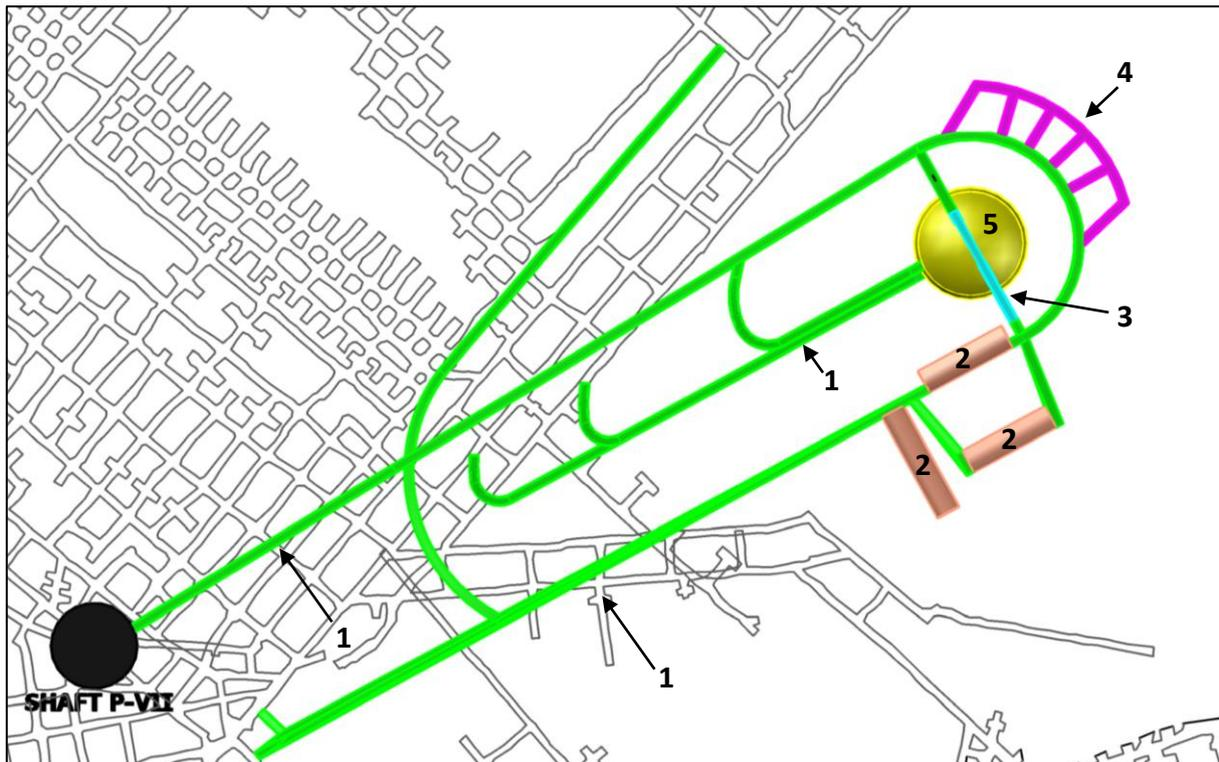
1 - ventilation/access ramp; 2 - functional chamber; 3 - office; 4 - Additional chambers (different usage possible); 5 - Main chamber
