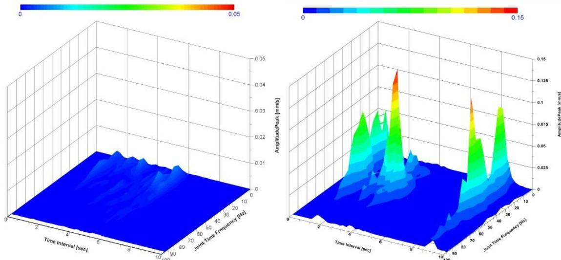
Figure 6.9. Relative seismic energy distribution after detonation of 25 faces- 1,465 kg left 22 faces- 1,470 kg
