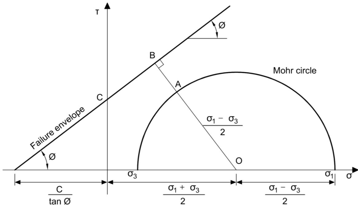
Figure 4.23. Mohr-Coulomb Failure envelope
