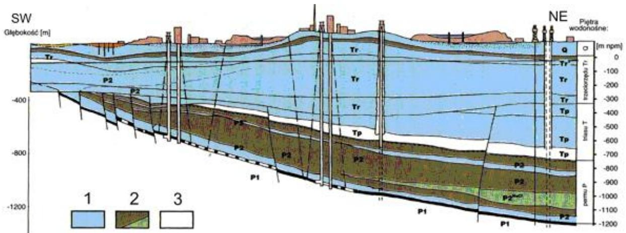
(1 – water deposits, 2 – impermeable deposits, 3 – impermeable but slightly saturated deposit)
