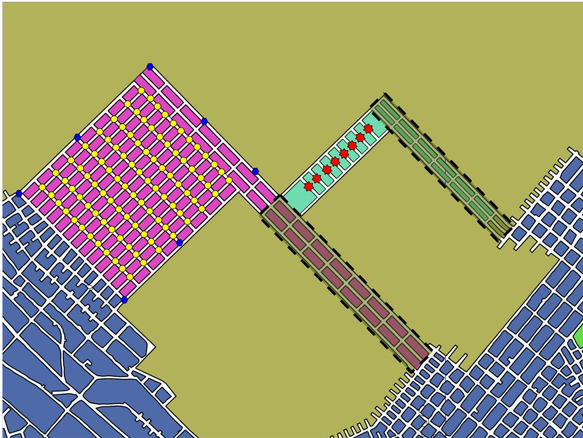
Figure 6.10. The geometry of the trial panel and location of monitoring devices
