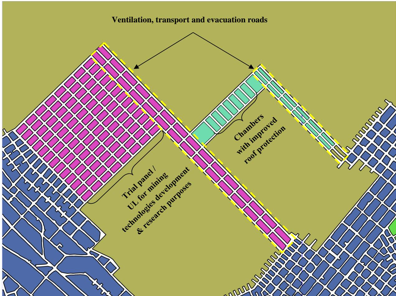
Figure 4.15. The geometry of the projected trial panel
