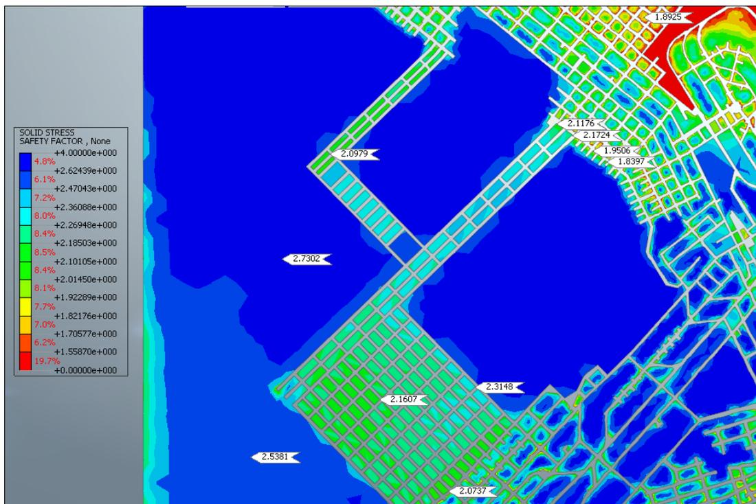
Figure 4.25. The distribution of safety factor in Conceptual Large-Scale Underground Laboratory (yellow frame)
