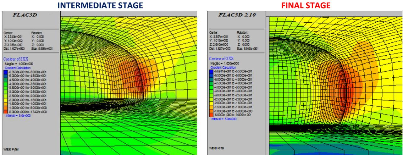
Figure 4.6. The contour of  $\sigma_{xx}$  stress (MPa)
