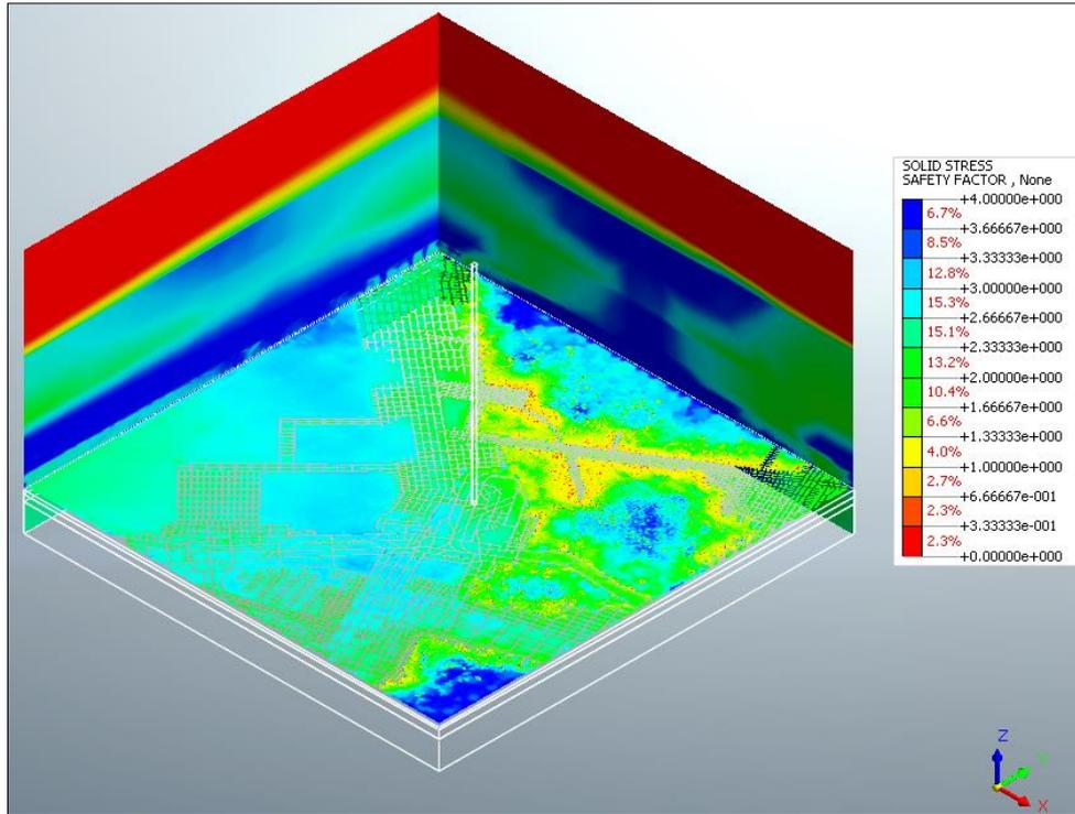
Figure 4.26. Cross-sections through the base of the trial panel (horizontal) and boundaries of a numerical model (vertical)
