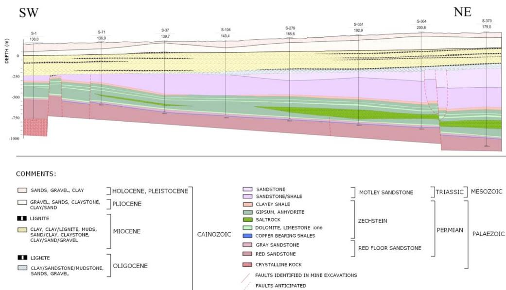
Figure 3.5. Geologic cross-section in Polkowice-Sieroszowice mine
