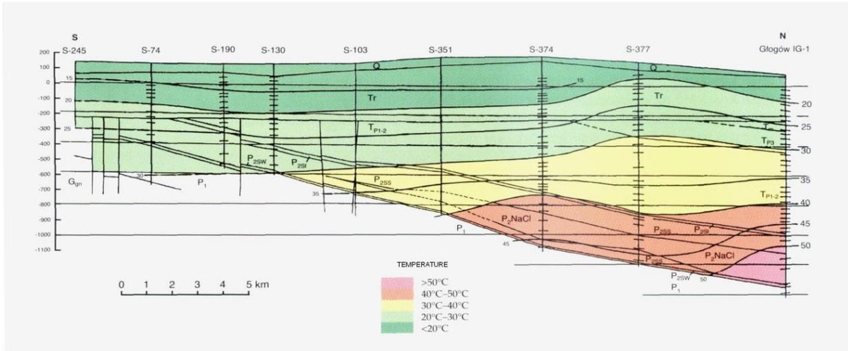
Figure 3.14. Geothermal cross-section of overburden in Polkowice-Sieroszowice area
