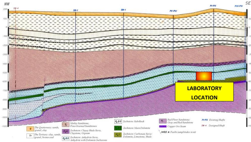
Figure 4.2. Overburden cross-section with the selected location of the underground laboratory
